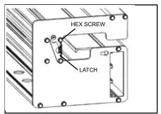
Loosen hex screw to allow Face Strip Retaining Latch to rotate out of the way. Insert Face Strip, reposition Latch and tighten screw.
