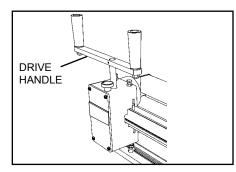
**6.** Using the handle, move the lacer head across the belt width at a smooth speed.
