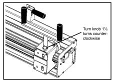
**5.** Return lacer head to end of lacer and turn adjusting knob 1½ additional turns counterclockwise.
